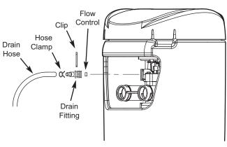
REMOVING DRAIN FITTING TO CLEAN FLOW CONTROL
