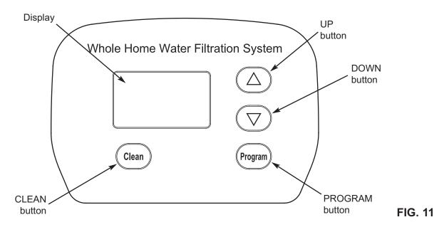
When the power supply is plugged into the electrical outlet, a model code and a test number (example: J2.0), begin to flash in the faceplate display. Then, 12:00 PM and the words "PRESENT TIME" begin to flash.
